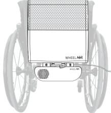
3. Ensure that the wheelAIR® logo is on the back side and that the fan box is aligned just below your seat.
