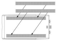
2. Determine whether your wheelchair support structure has hook or loop Velcro and remove the loop Velcro strips from the wheelAIR® backrest cushion if necessary.
