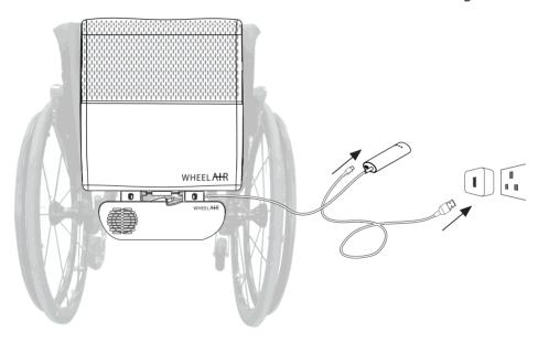
Charging is taking place when the LEDs are pulsing blue.
